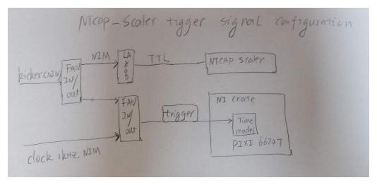
Scaler trigger configuration. We use the precise kicker signal generated by the new timing module. We split this signal into two paths: one is directly sent to the scaler channel 11 of NTCAP. The other path is combined with the Clock signal using a logical OR operation, then converted into a TTL signal, and sent to the trigger channel of the NTCAP.
