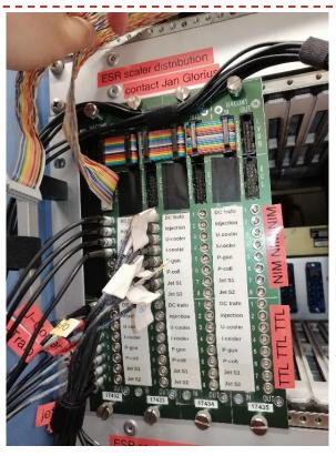
The new injection signal is from the time module at ESR. The new time module provide precise time of the kicker signal.
