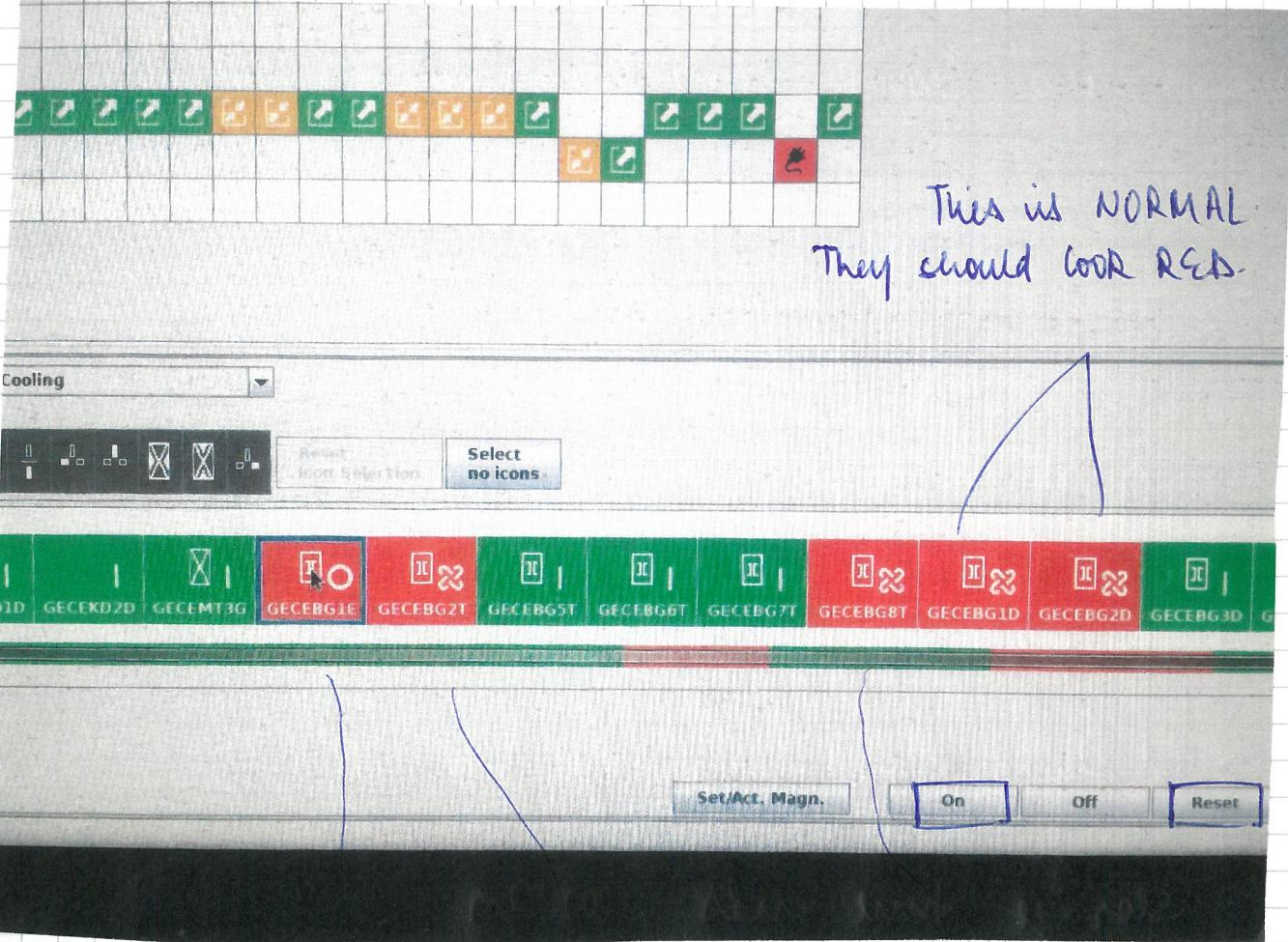
Aj 1) GECEBG1E, GECEBG2T & GECEBG8T are RED which means, electron cooler is BROKEN
