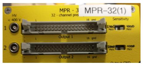
MPR-32 (1) has been found untouched after the experiment with the 1GeV sensitivity setting. At this point MPR-32 (2) was already in use again elsewhere and cannot be checked for its setting anymore.
