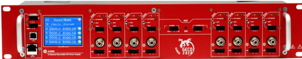
Fig. 4: R14xxET Front panel (8 channel)
