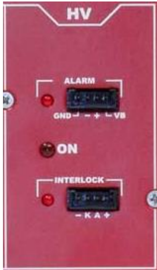
Fig. 12: HV Status control panel
