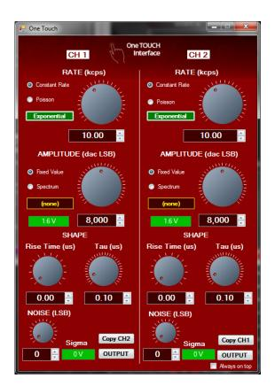
Action 1: set the RATE to "Poisson", and change the rate value to 2 kHz.
