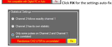
Note: By default both channel 1 and channel 2 start with the same seed. Remember to randomize the channel 2 LFSR to get uncorrelated distributions. Click FIX to let the GUI auto-fixes the settings.
