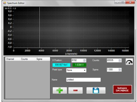
Point the cursor on the diagram, and double click to add a line. The x-axis is in counts unit. In the pop-up write the corresponding value of height. 65535 is the maximum value allowed.
