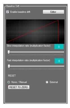
Click on "Enable baseline drift" to enable the linear baseline drift. The emulator will sum the desired baseline drift to the signal output.
