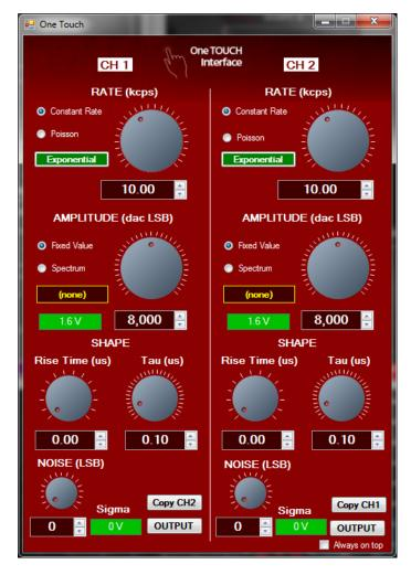
The main parameters for the signal generation can be set either through the virtual knob, the underlying box, or the green box.
